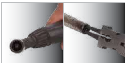
Welding Gun Nozzle filled with weld splatter
