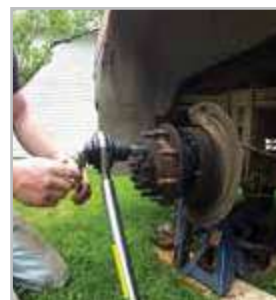
Torque multiplier used for lug nuts
