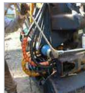
Torque multiplier used for machine nut tightening
