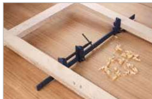
Duo Bar used for internal clamping
