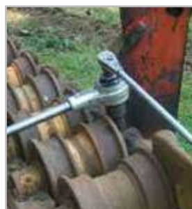
Torque multiplier used on tracks
