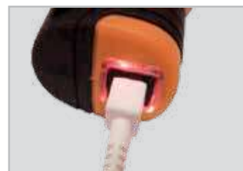
Red light show charging on & Green light shows charging complete
