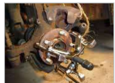
3 Jaw Puller used for removing tyre hub
