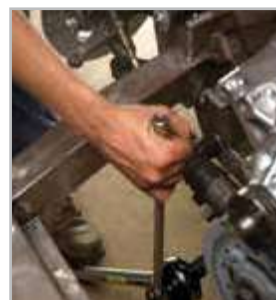
Torque multiplier used in inaccessible areas
