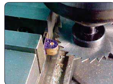
SlittingSawArborbeingusedforaslittingoperation on a job being worked upon on a milling machine
