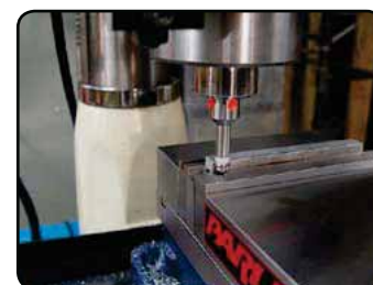
Edge Finders being used to locate the edge of a job held in a milling vice
