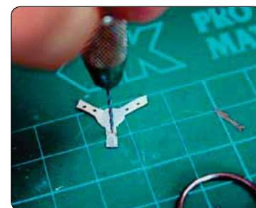
PinVicebeingusedtoholdadrillforhand-drilling on an electronic component
