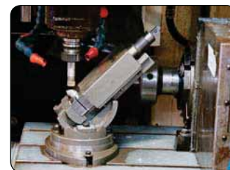
The Angular Machine Vice being used for 45° face milling
