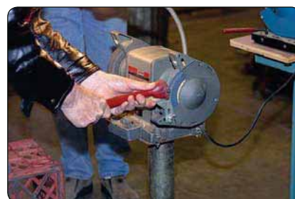
Dressing the wheel of a Bench Grinder
