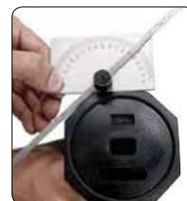
Depth Gauge with Protractor being used for angular measurements
