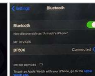
To activate Bluetooth, press and hold the ON button for switching on the Bluetooth mode and connect to "BT500" from your phone
