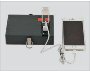
Rechargeable & removable battery pack can also be used as a power bank
