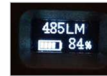
OLED screen real time display of Lumens and battery level
