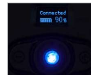
To activate Bluetooth, press and hold the ON button for switching on the Bluetooth mode and connect to "BT500" from your phone
