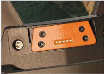
Battery Level Indication on battery pack va 5 LED battery level indicator. Each Led indicates 20% charge
