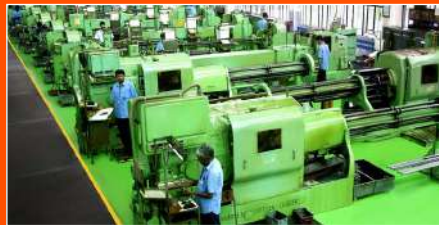
Multi-Spindle Turning Machines - Davenport's for high volume production & concentricity
