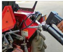
Without Swivel - Twisting of hose
