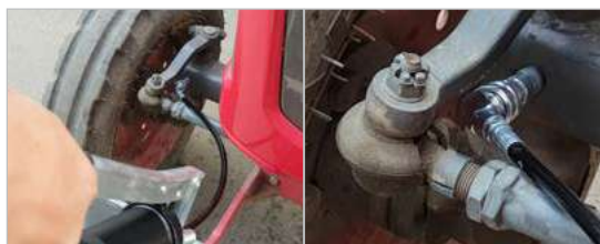
Convenient access into narrow, inaccessible greasing joints
