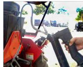
With Swivel - No Twisting of hose
